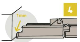
Clip and slide the SUNDIY mechanism onto the clip, leaving a gap of about 1mm between the beginning of the structure and the mechanism (closed).
