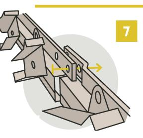
Join the two mechanisms using rivets (or bolts), taking care to position the completely straight part in front of the slightly bent part.
